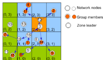
Fig. 1: Zone structure and multicast session example.
